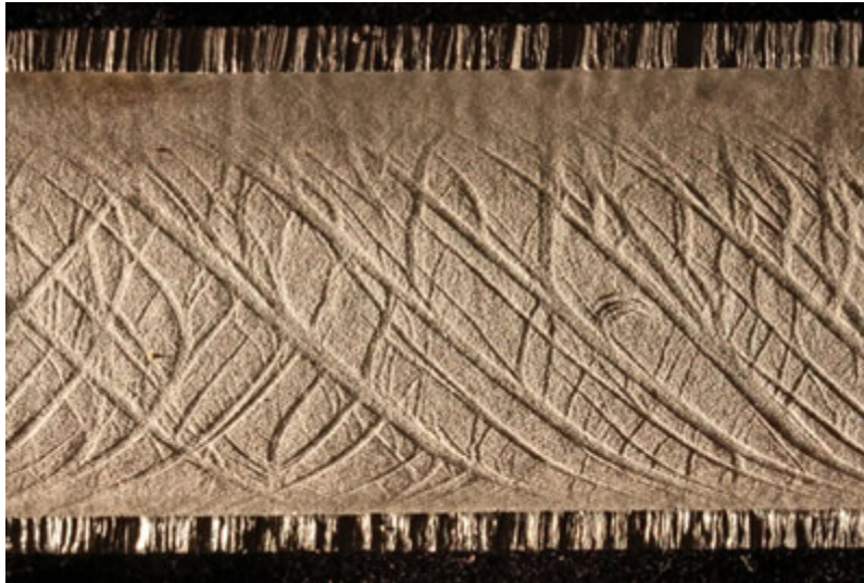
Figure 11. Close-up view of pipe internal surface after cleaning
